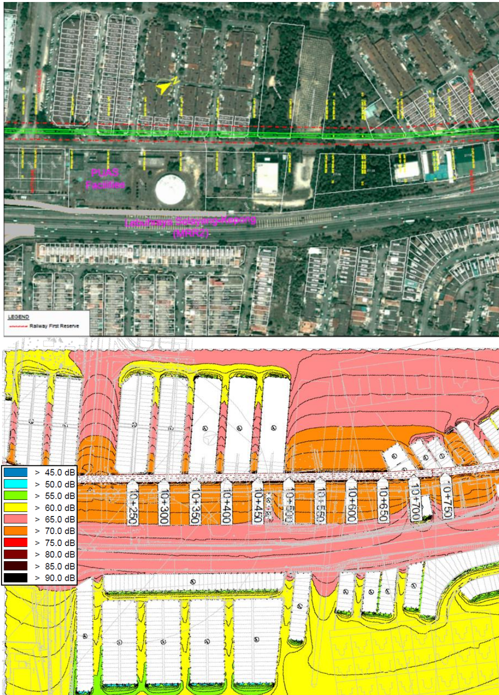
Figure 7: Noise contours ( L_{\max} levels) on grade for transit trains from 3D noise modelling of trains pass by on elevated viaducts to the environment
