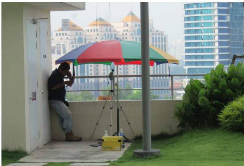
Figure B-16: Example of unacceptable monitoring in progress with sound level meter placed under an umbrella (apparently for weather protection)
